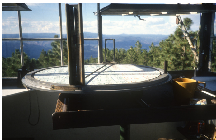
Fig. 13 The Alidade at Bear Mountain. Regardless of plan, the central feature of any lookout is the alidade, which is affixed to a stand or cabinet. The standard alidade is the Osborne firefinder.
